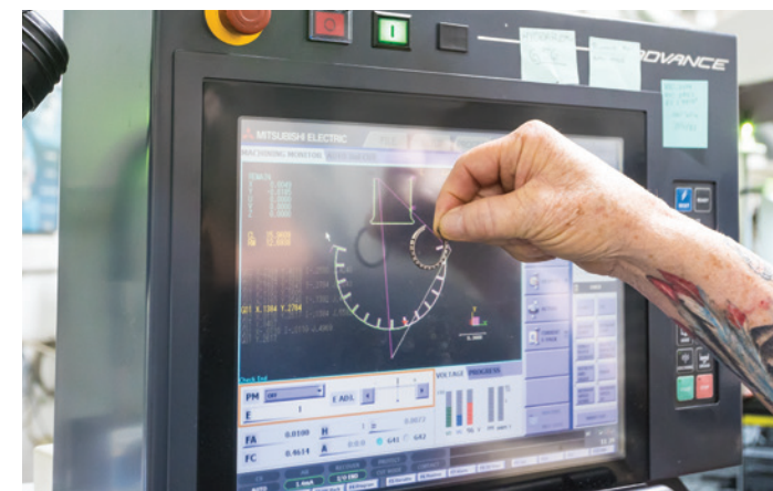
The Mitsubishi NA1200 wire EDM is unique because it can use a thinner wire for even tighter tolerances.
