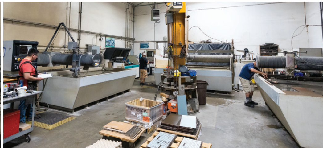
Milco has three Omax abrasive waterjets. Steve was an early adopter of the technology. He is of the opinion that the Omax software is the best in the business and well ahead of the competition. The trio of machines run practically non stop.
